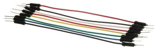
Fig. 5. Connecting wires - Image source India-mart
