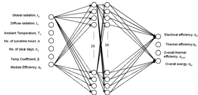
Figure 1(b): Input, output and hidden layers of ANN for double pass air collector.
