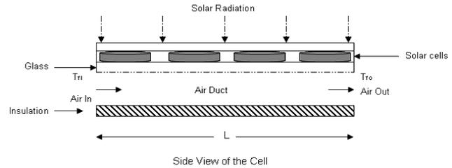
Figure 3(a): Schematic diagram of hybrid photovoltaic thermal single pass air collector.
