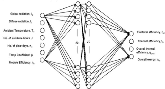
Figure 1(a): Input, output and hidden layers of ANN for single pass air collector
