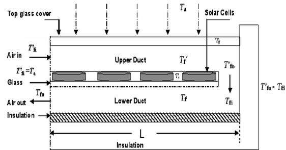
Figure 3(b): Schematic diagram of a hybrid photovoltaic thermal double pass air collector
