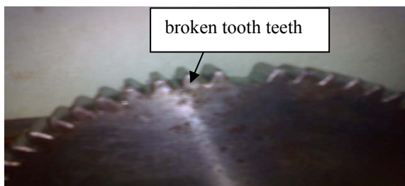
Figure 3: Gear with One Tooth Broken or Missed
