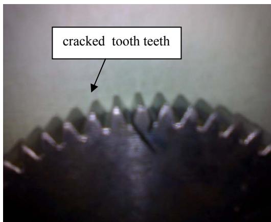
Figure 4: gear with crack on one tooth
