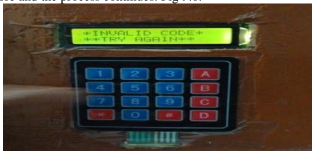
Figure 13.0. Incorrect password entry.
