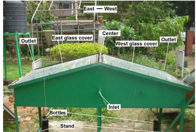
**Figure 1:** A photograph of double slope solar still.
