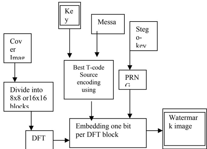
Figure 2.1: “The block diagram for watermark embedding process”
