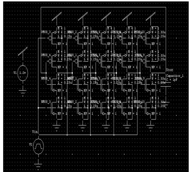
Figure 14: “Schematic Circuit of proposed VCO with voltage applied to both PMOS and NMOS transistors”
