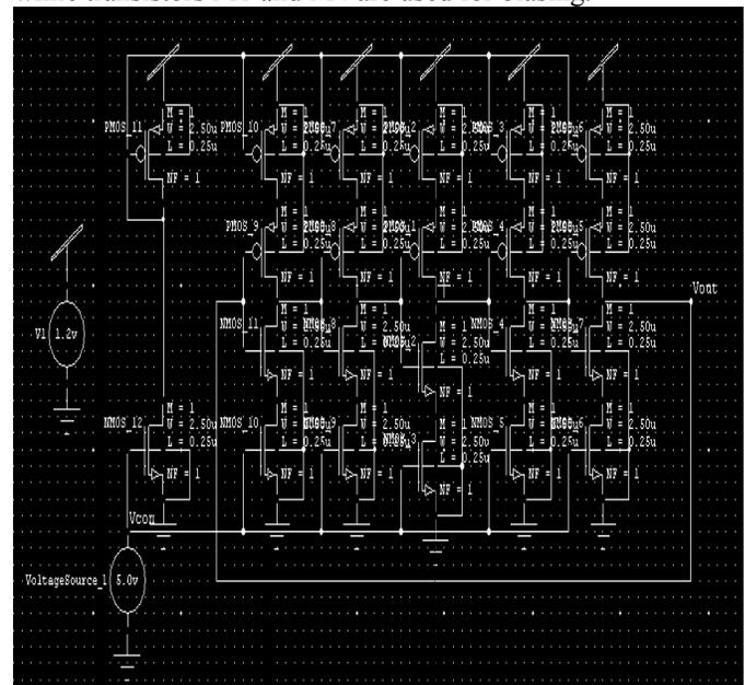
Figure 2: “Schematic circuit of Current Starved VCO”
