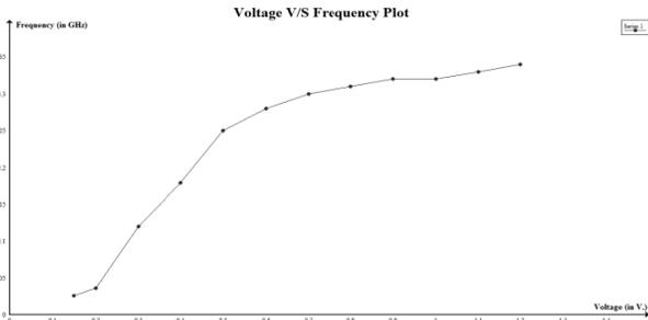
**Figure 10: "Voltage vs. Frequency Plot of VCO with PMOS Transistor Diode Connected"**
