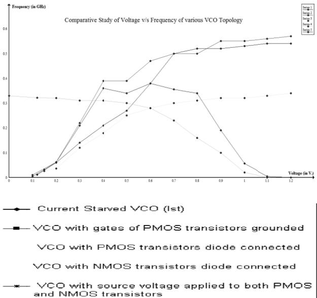
**Figure 17: "Comparative analysis of Voltage Vs Frequency of various ring topology VCO"**
