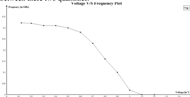
Figure 13: “Voltage vs. Frequency Plot of VCO with NMOS Transistor Diode Connected”
