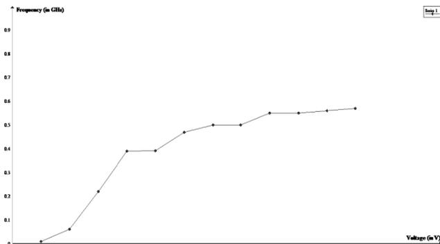
**Figure 7: “Voltage vs. Frequency Plot of VCO with gates of PMOS transistors grounded”**
