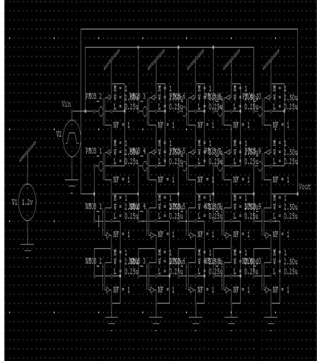
**Figure 11: "Schematic Circuit of proposed VCO with NMOS transistors diode connected"**
