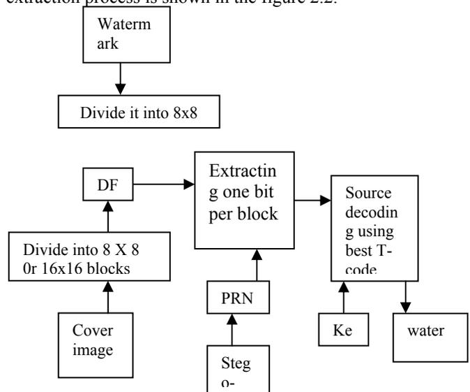
Figure 2.2: “The block diagram of the watermark extraction process”
