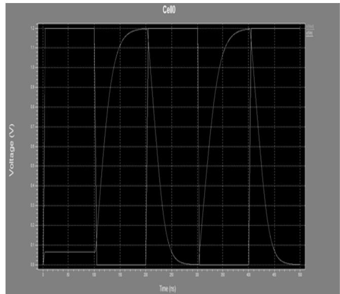
Figure 15: “Simulated results of proposed voltage applied to both PMOS and NMOS transistor VCO pulse input voltage”
