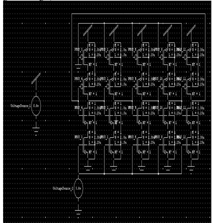
Figure 5: “Schematic Circuit of proposed VCO with gates of PMOS Transistors Grounded”
